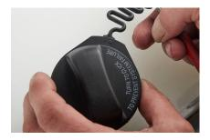
Unhook the catch strap from the fuel door and remove the tank cap together with the catch strap.
