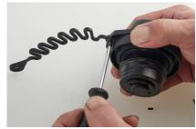
Use a small Torx or Phillips screwdriver (max. 2mm diameter) to push the pins slightly forward from the bottom side.
