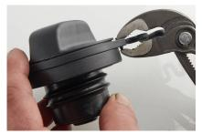
A small water pump pliers is best suited for pushing the pins through. Be careful when pushing them through, the pins deform quite easily.
