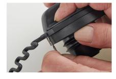
If they have come loose, you can press the pins through from the inside on a table edge or similar with a 2mm drill. They only need to be pushed through until they are just inside the top of the fastener.
