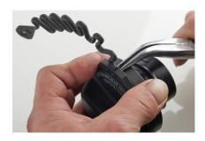
Insert the new catch strap into the tank cap. If the pins have been pushed through too far and have fallen out, a telephone plier or tweezers will help to reattach them.
