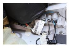
There are cables harnesses below the insulatuion mat. Tape them to the floor to prevent contact with the Isofix-Bracket.
