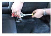
Undo the belt lock mounting screw.
