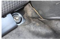
On the other side the Isofix bracket is mounted to the stud using the new supplied nut. Because the nut is self-locking crimped, tightening is relatively difficult.
