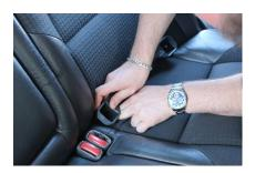
We recommend to use a cover which is simply pressed on the ISOFIX brackets and speads the upholstery to make the brackets reachable. They also prevent the upholstery from being damaged when the child seat engages.
