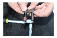
The kit includes a new longer screw. Mount the Isofix bracket and the belt lock together with the new screw.
