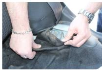
Pull the insulation mat out from under the sill cover and fold it aside.
